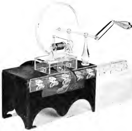
Figure 17.—MOREY AND JOHNSON sewing machine, 1849. Below: The machine is marked with the name of its maker, Safford & Williams. The number 49 is a serial number. Missing parts have been replaced with plastic. (Smithsonian photo 48400; brass plate: 48400-H.)
